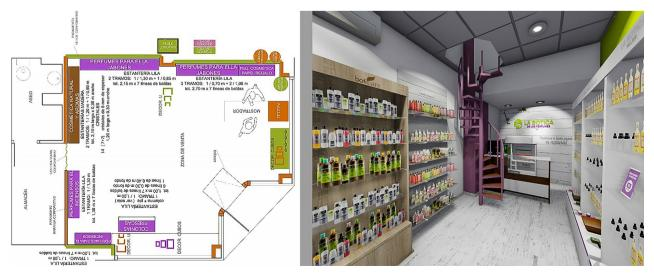
Figure 2. Graphic outcomes corresponding to traditional CAD (left) and BIM (right) techniques (LBP file)
