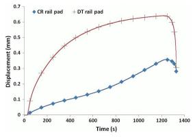
Fig. 4. Time-displacement curves measured in the static test at loads of 20–95 kN
