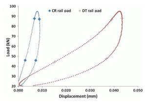
Fig. 5. Load-displacement curve of the dynamic test
