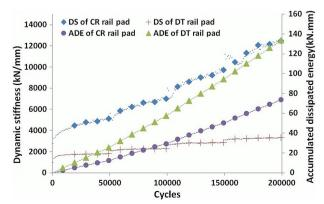
Fig. 7. Long-term analysis of dynamic stiffness (DS) and accumulated dissipated energy (ADE)
