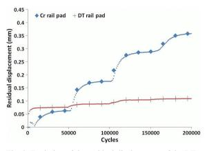
Fig. 8. Evolution of the residual displacement of the DT and CR rail pad
