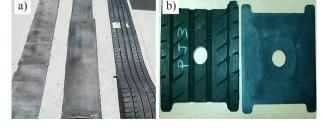
Fig. 1. a) Tire layers: inner (left), middle (center) and outer (right). b) Rail pad made of deconstructed EOL-tires (left); commercial rail pad made of crumb rubber particles (right)
