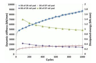
Fig. 6. Dynamic stiffness (DS) and dissipated energy (DE) for DT and CR rail pads
