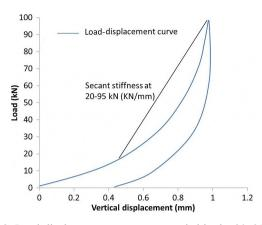
Fig. 2. Load-displacement curve, as recorded in the 20–95 kN static test
