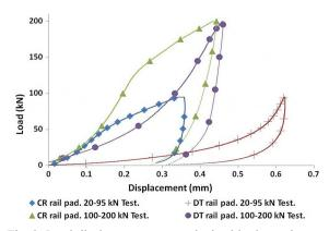
Fig. 3. Load-displacement curves obtained in the static tests
