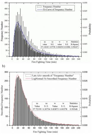
Fig. 1. Frequency histogram for urban fire data of Jiangxi Province from 2000 to 2010 along with the lognormal distribution curve: (a) Original data, (b) Five-points smooth data
