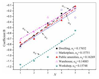
Fig. 7. Regression curve of coefficient B of power law and fire fighting time interval (N) with different sites
