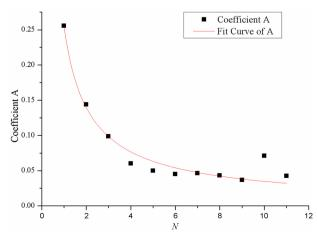
Fig. 3. Regression curve of coefficient *A* of power law and fire fighting time interval
