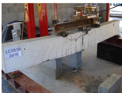
Fig. 3. Test beam after failure
