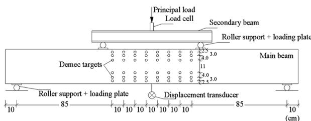
Fig. 2. Set-up for testing beam specimen (Bernardo et al. 2014)
