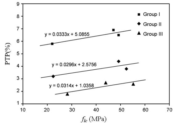
Fig. 8. Influence of concrete strength on the PTP
