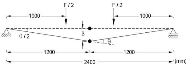
Fig. 6. Global plastic mechanism and plastic rotation
