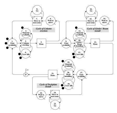
Fig. 4. SCHEME for steel structure construction
