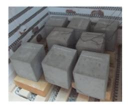
Figure 2. Arrangement of specimens inside the furnace
