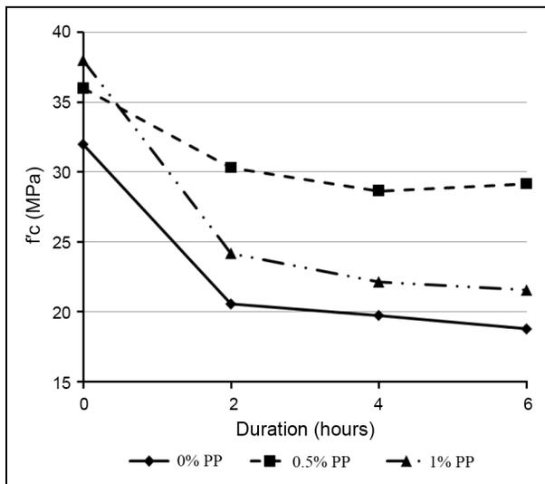
Fig. 4. Compressive strengths for 400 °C
