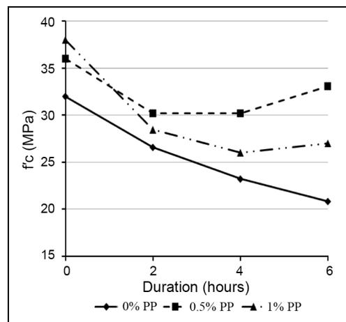
Fig. 3. Compressive strengths for 200 °C
