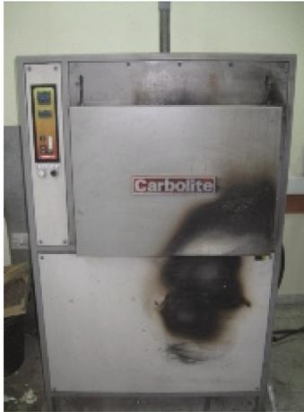
Fig. 2. The furnace used for heating the specimens
