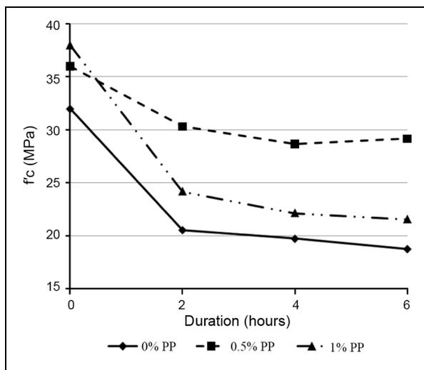
Fig. 5. Compressive strengths for 600 °C
