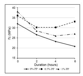
Fig. 3. Compressive strengths for 200 °C
