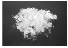
Fig. 1. Polypropylene fibers used
