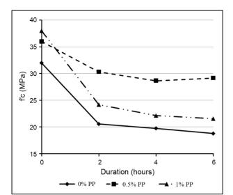
**Fig. 4.** Compressive strengths for 400 °C
