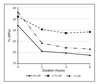
Fig. 5. Compressive strengths for 600 °C
