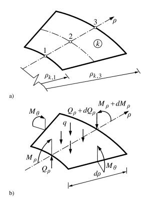
**Fig. 1.** The finite element of a round plate (a); the positive directions of internal forces (b)
