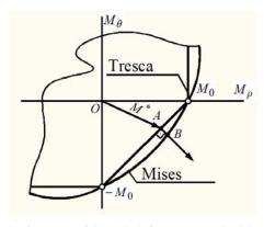
**Fig. 3.** The fragment of the switch from Tresca plasticity conditions to Mises plasticity conditions
