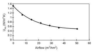
**Fig. 8.**  $U_{eq}$  for different air flow rates (Southall and McEvoy 2006)
