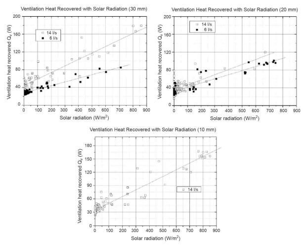
Fig. 10. Ventilation heat recovered vs. incident solar radiation for different air gap widths (Southall and McEvoy 2006)
