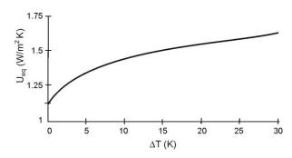
Fig. 9.  $U_{eq}$  in function of temperatures difference (indooroutdoor) (Park 2003)
