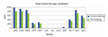
Fig. 11. Monthly heat losses through ventilation with and without pre-heating of ventilation air
