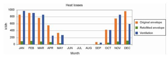
Fig. 6. Monthly heat losses through the envelope and heat losses through ventilation
