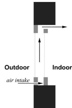
Fig. 7. Ventiladed double window (Arons and Glicksman 2003)
