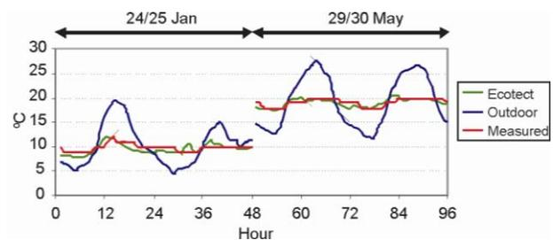
**Fig. 4.** Local measurements vs. ECOTECT simulations
