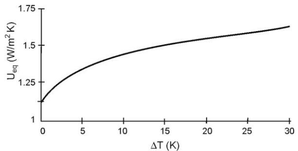
Fig. 9.  $U_{eq}$  in function of temperatures difference (indoor-outdoor) (Park 2003)
