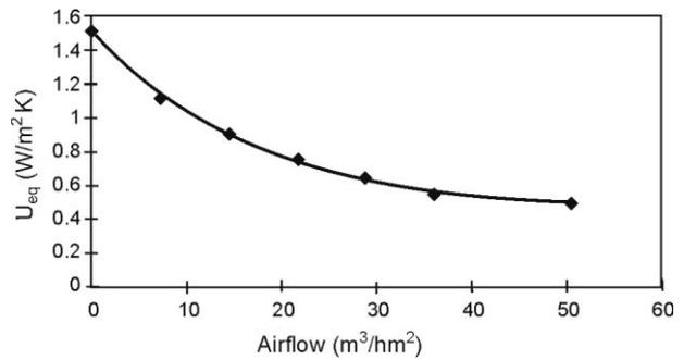
Fig. 8.  $U_{eq}$  for different air flow rates (Southall and McEvoy 2006)
