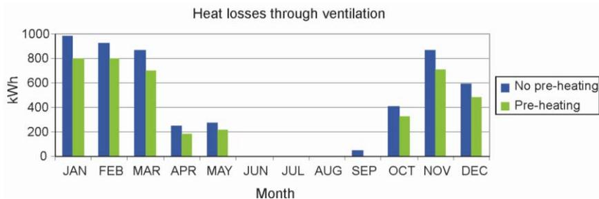
Fig. 11. Monthly heat losses through ventilation with and without pre-heating of ventilation air
