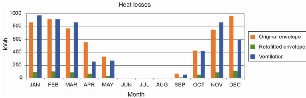
Fig. 6. Monthly heat losses through the envelope and heat losses through ventilation
