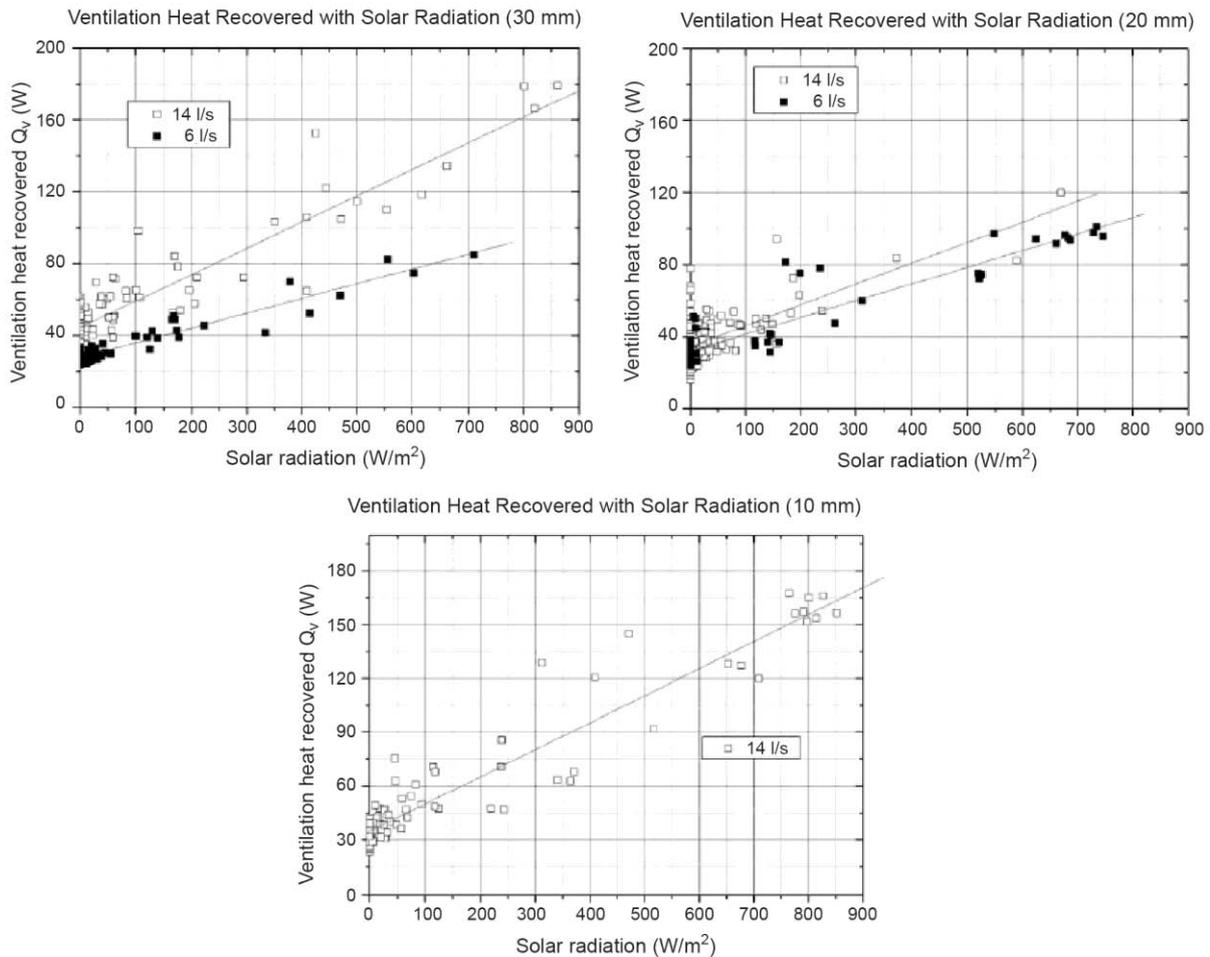
Fig. 10. Ventilation heat recovered vs. incident solar radiation for different air gap widths (Southall and McEvoy 2006)
