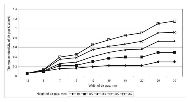
Fig. 3. The measured thermal conductivity values of vertical gaps of various widths and lengths
