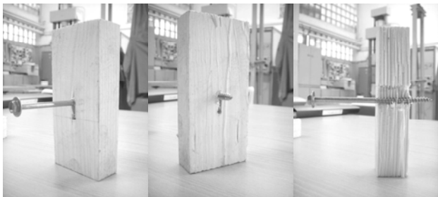
Fig 5. Arrangement of screws in specimen at tests for determination of their withdrawal capacity
