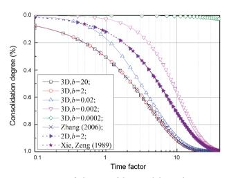
Figure 3. Verified curves of the consolidation degree
