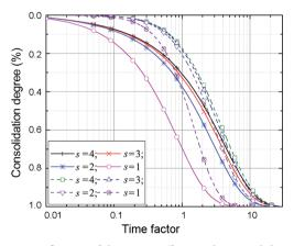
Figure 10. Influence of the smear effect on the consolidation degree. The solid lines and dashed lines represent b = 2 and b = 0.02, respectively
