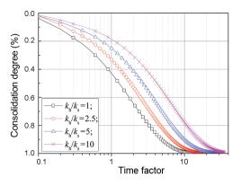
Figure 9. Effect of permeability coefficient of smear area on degree of consolidation
