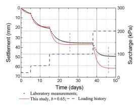
Figure 12. Comparison curves of settlements versus time between experiment and calculation
