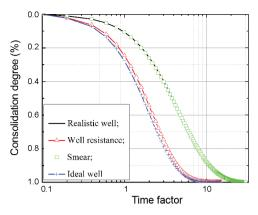
Figure 11. Influence of the smear effect and the well resistance on the consolidation degree
