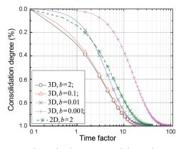
Figure 7. Relationship between consolidation degree and time under different drainage conditions of the foundation top surface, The solid lines and the dashed line represent the results of considering and not considering the top drainage
