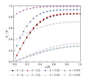
Figure 5. Relationship between excess pore water pressure and depth at different consolidation times and top water drainage capacities, The solid lines and dashed lines represent  $T_h = 1.4$  and  $T_h = 7$ , respectively
