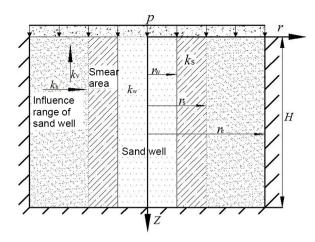
Figure 1. Vertical-drain foundation model
