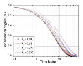
Figure 8. Influence of well resistance on consolidation degree
