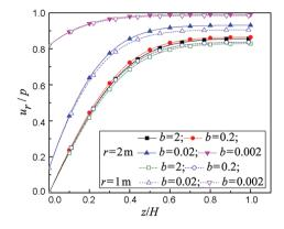
Figure 4. Relationship between excess pore water pressure and depth at different horizontal locations and top water drainage capacity
