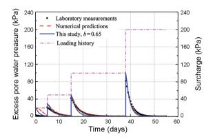
Figure 13. Variation of excess pore water pressure versus time obtained by different methods
