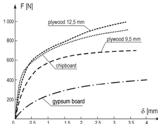
**Fig 11.** Deformability of sheathing to framing connectors for different sheathing material
