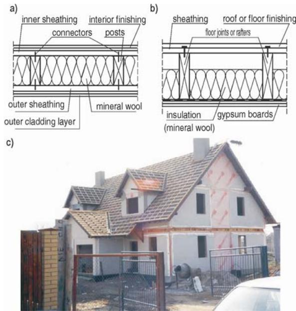
**Fig 1.** Typical cross-section of the wood-framed structures and a building under construction: a) wall diaphragms, b) floor and roof panel, c) a building under construction
