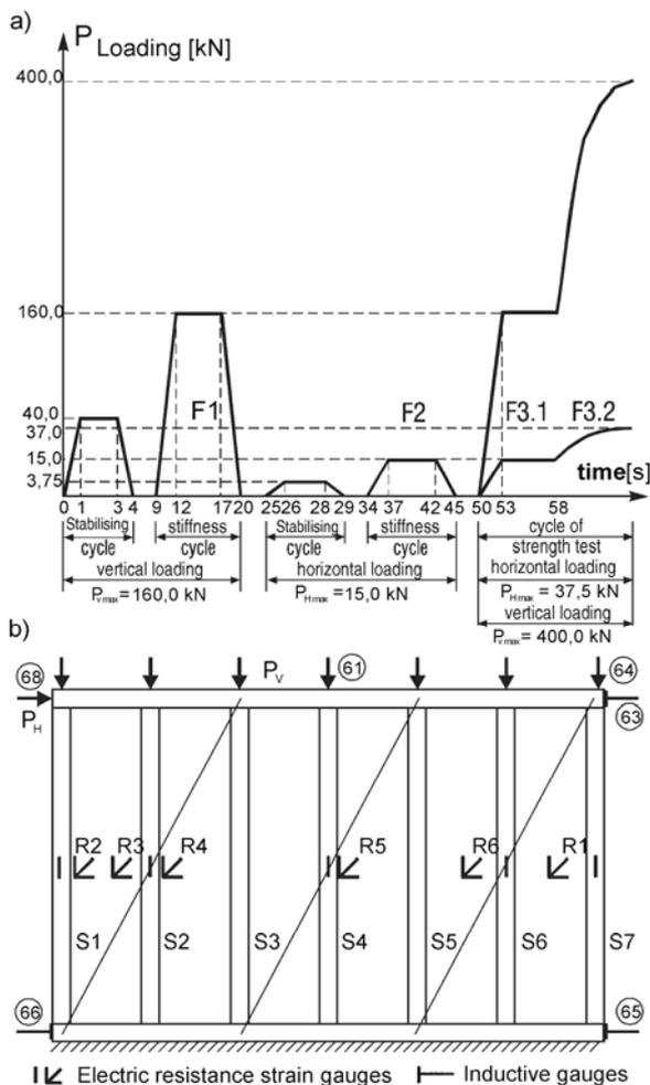
Fig 4. Scheme of application and phases of loading: a) phases of loading, b) strain gauges and inductive gauges location
