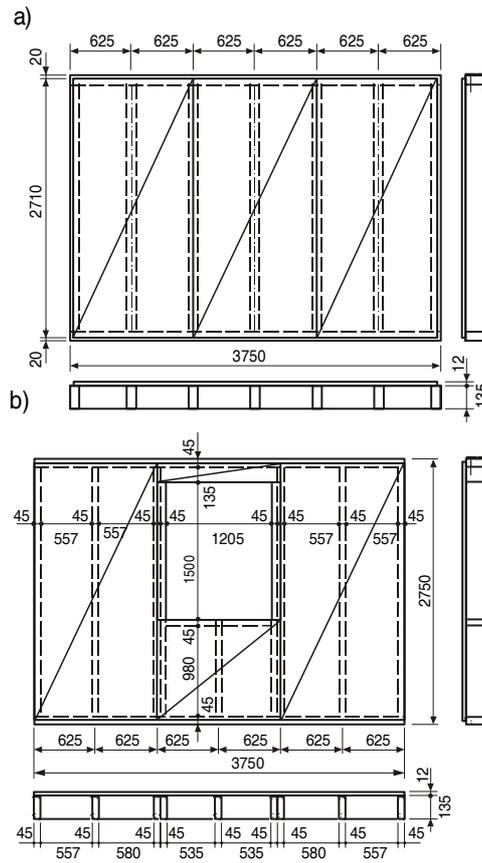
**Fig 3.** Experimentally investigated wall panels: a) full wall panel A, b) perforated wall panel B
