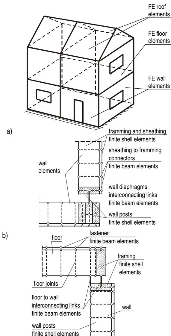
**Fig 10.** Modelling the building and joints a) walls at the corner, b) floor to wall
