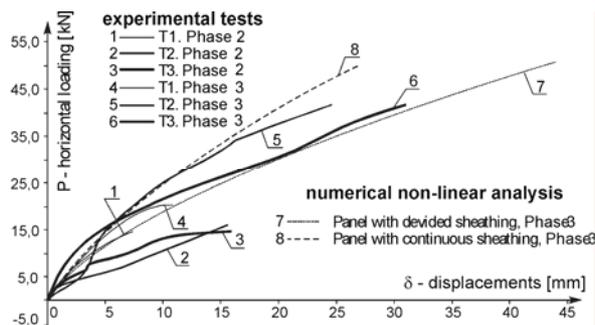
**Fig 12.** Experimental and analytical characteristics of wall deformability
