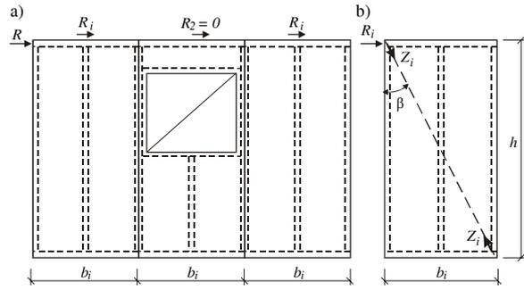
**Fig 6.** Distribution of internal forces within diaphragm: a) lateral load distributed in the wall, b) lateral load distributed within the single panel
