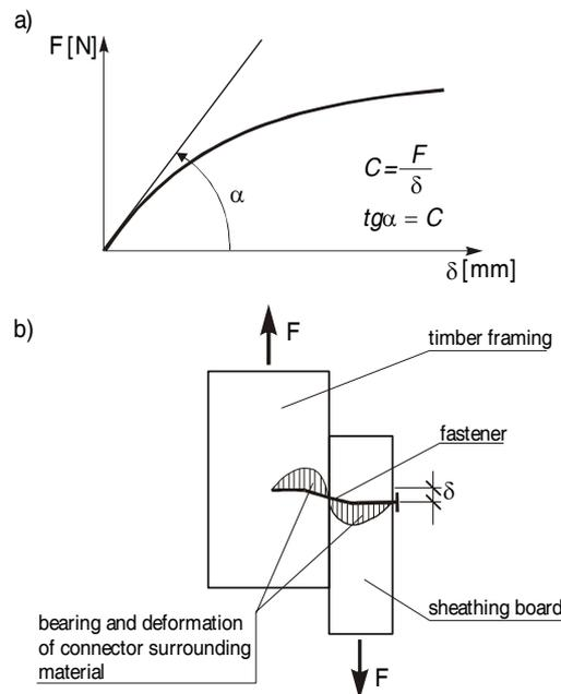
Fig 5. Behaviour of fastener and response of surrounding material: a) load-slip characteristic, b) behaviour of fastener surrounding material
