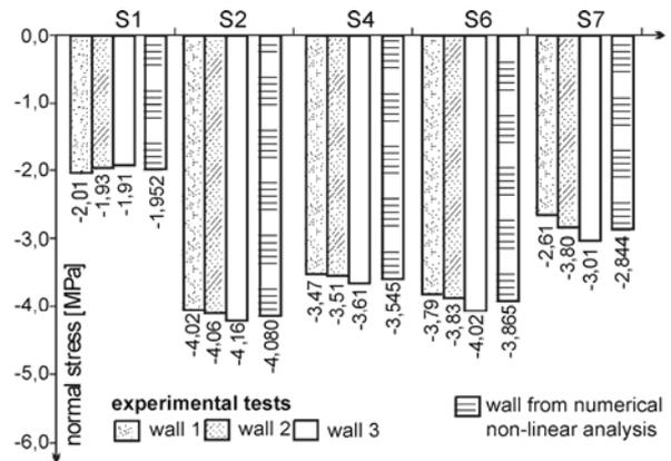
**Fig 13.** Diagram of stressing in the studs of walls without opening
