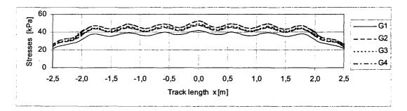
Fig 3. Diagram of stress variability along track, under rail axis, at depth of 0,50 m, depending on type of force distribution under sleeper surface
