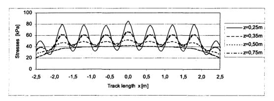
Fig 5. Distribution of stresses at subgrade depth under the most heavily loaded sleeper
