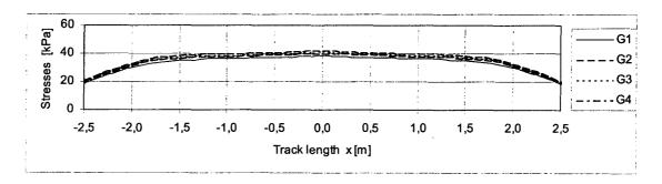
Fig 4. Diagram of stress variability along track, under rail axis, at depth of 0,75 m, depending on type of force distribution under sleeper surface
