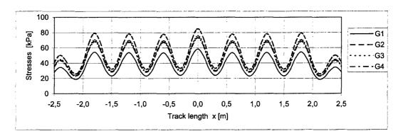
Fig 2. Diagram of stress variability along track, under rail axis, at depth of 0,25 m, depending on force distribution under sleeper surface
