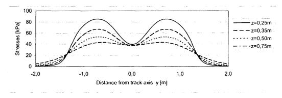
Fig 7. Diagram of stress variability in subgrade at different depths in cross-section of track for scheme G2
