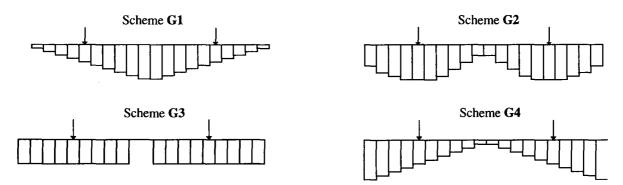
Fig 1. Schemes of distribution of stresses transferred through sleepers to ballast
