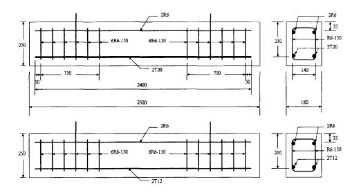
Fig 1. Design for B1 and F series specimens (top: B1; bottom: F1 to F3)
