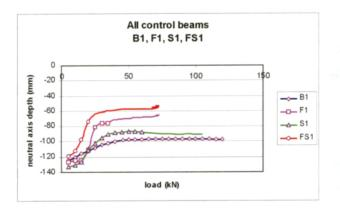
Fig 14. Neutral axes for control beams
