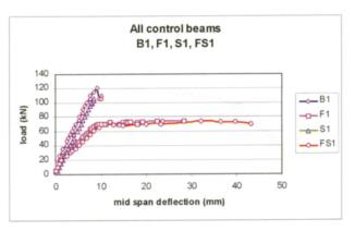
Fig 10. Load-deflection curves for control beams
