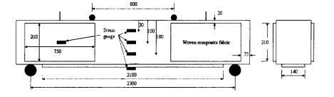
Fig 3. Loading and instrumentation details for FS series specimens
