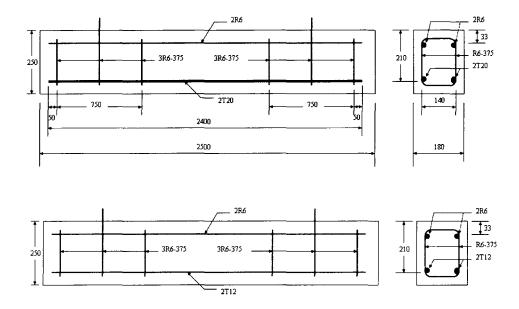
Fig 2. Design for S and SF series specimens (top: S1 to S3; bottom: FS1 to FS3)
