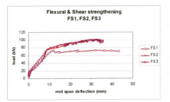
Fig 13. Load-deflection curves for FS series beams
