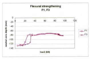
Fig 15. Neutral axes for F1 and F3
