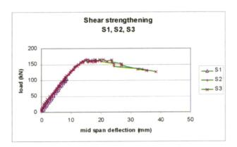
Fig 12. Load-deflection curves for S series beams
