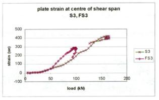
Fig 18. Strain of side FRP plate
