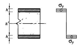
Fig 4. Three-layered bending plate cross-section
