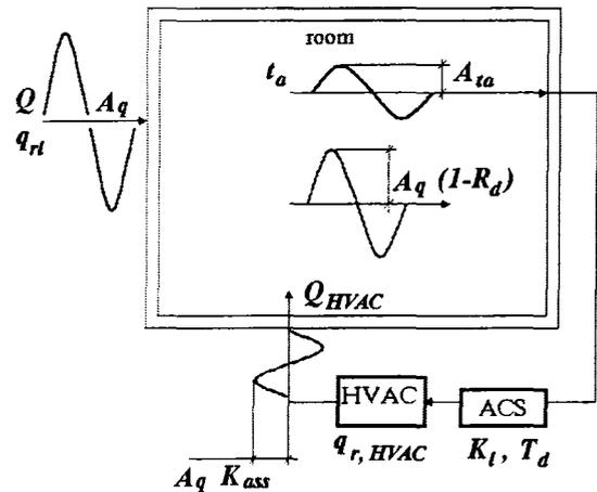
Fig 2. The pattern of transient processes in the system «room-HVAC and ACS-systems» in condition of the unsteady duties
