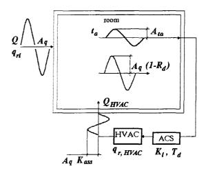
Fig 2. The pattern of transient processes in the system «room-HVAC and ACS-systems» in condition of the unsteady duties
