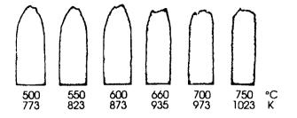
Fig. 2. Character of failure of the stainless steel samples (10% Cr, 95% Ni) in raised and high temperatures
