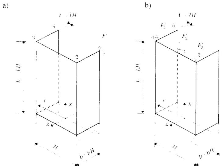
Fig. 3. Thin-walled beam with  $U$ -type cross-section:
