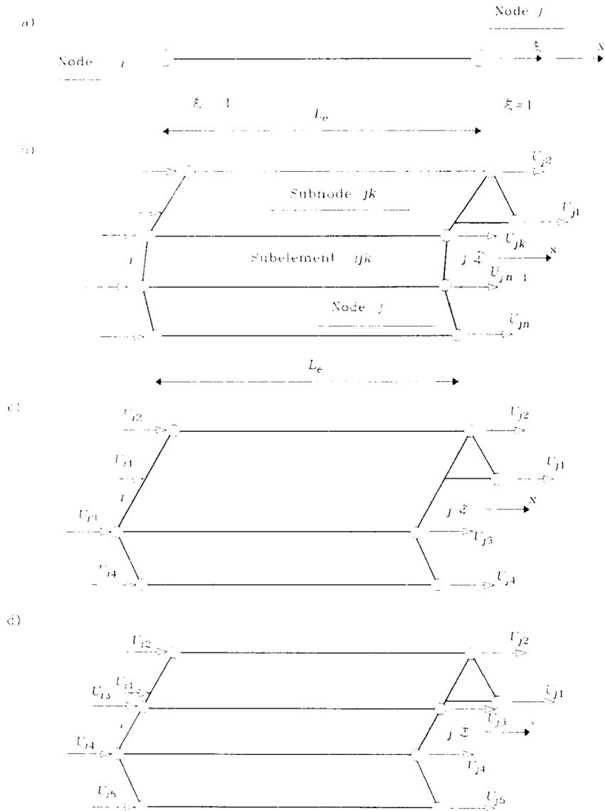
Fig. 1. Semi-analytically based primary finite elements of a thin-walled beam:
