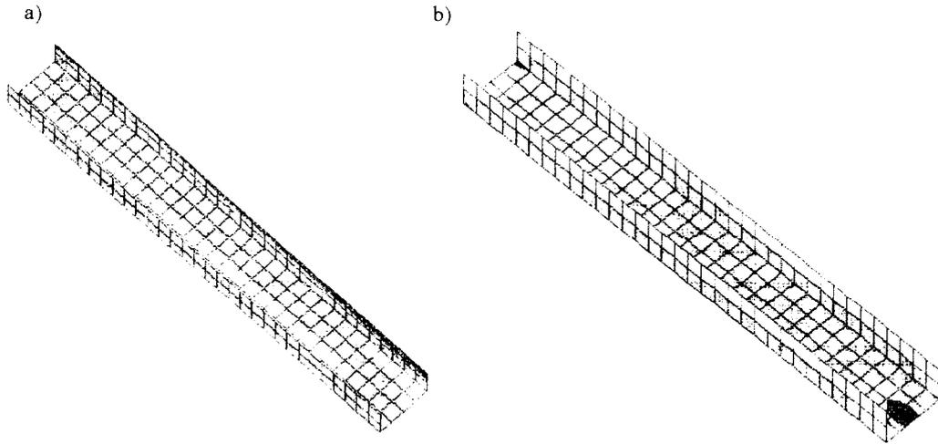
Fig. 5. Space distribution of nondimensional stresses  $\bar{\sigma}_x$  obtained by shell model:
