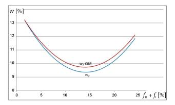
Figure 14. The changes of the moisture trend line in the middle of the soil sample before and after the CBR test with regard to the fine fraction content
