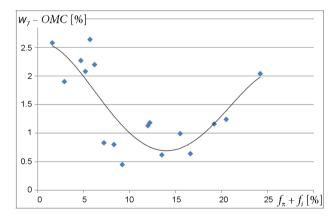
Figure 8. Increase of the moisture content as a function of the fine fraction content
