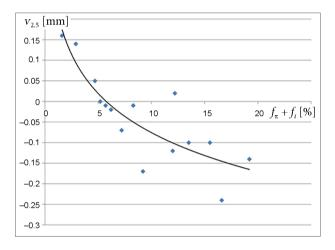
Figure 10. The dependence between annular surcharge rings displacement and the fine fraction content for penetration depth of 2.5 mm
