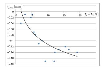
Figure 9. The dependence between maximum downward displacement of the annular surcharge rings and the content of fine fraction
