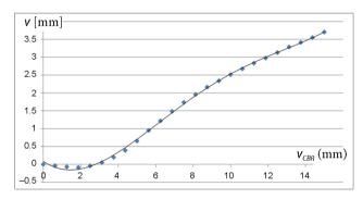
Figure 15. The dependence between the indentation of the press piston  $v_{CBR}$  and the displacement of annular surcharge rings v
