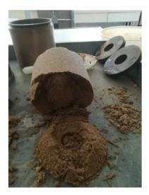
Figure 3. The view of the soil sample after the CBR test
