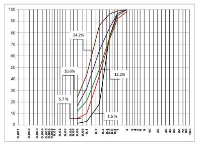
Figure 1. The grading curves of selected soils
