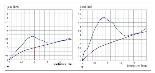
Figure 12. Corrected penetration graphs of soil samples (a) fine fraction content: 5.7% (b) fine fraction content: 12.0%
