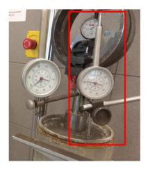
Figure 4. The location of the annular surcharge ring displacement sensor in the CBR loading press
