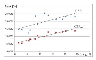
Figure 11. The dependence between the fine fraction content and the CBR value
