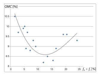
Figure 6. The dependence between optimum moisture content and the fine fractions content
