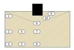
Figure 2. The distribution of moisture measurement points in the cross-section of soil samples
