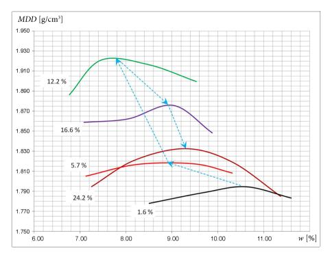
Figure 7. Changes of soil compactibility curves with different content of fine fractions
