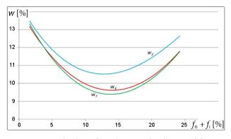
Figure 13. The dependence between the changes of the moisture trend line in the middle of the soil sample and the fine fraction content
