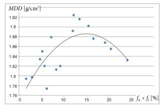
Figure 5. The dependence between the maximum dry density and the content of fine fractions
