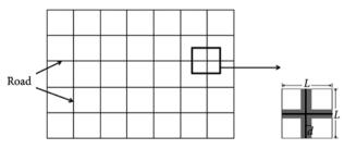
Fig. 6. Square grid layout of road network. Within each unit area, the edge effect of roads is in gray strips
