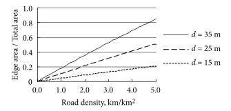
Fig. 7. Relationship between the edge area/total area ratio and road density with varying edge widths
