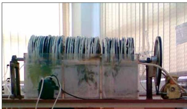
Fig. 1. The RBC with developed biofilm after start-up
