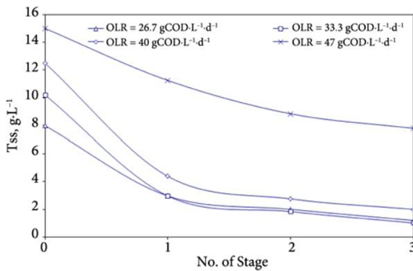
Fig. 4. TSS concentration profiles in different stages of RBC at various OLR
