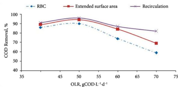
Fig. 6. COD removal with various OLR in RBC, with extended surface and recirculation at HRT of 24 h
