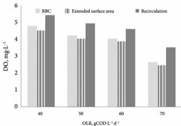
Fig. 5. DO level with respect to OLR for RBC, extended surface and recirculation
