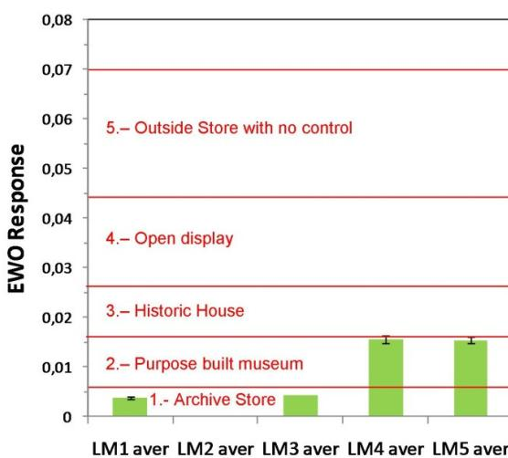
**Fig. 2.** EWO dosimeter responses ( $\Delta\text{Light absorbance}$ ) obtained in the five indoor locations in the LTMCM
