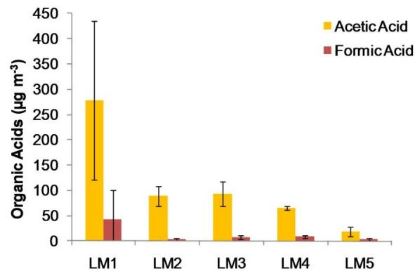
**Fig. 5.** Organic acids (acetic and formic acids) concentration measured in the LTMCM. Values represent the average from two parallel samplers. For abbreviations and location characteristics see Table 1
