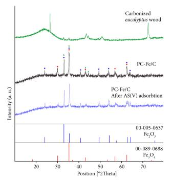
Figure 1. XRD patterns of the PC-Fe/C adsorbent prepared with eucalyptus wood biotemplate
