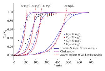
Figure 4. Effect of influent concentration on breakthrough curve for As(V) adsorption removal by the PC-Fe/C adsorbent prepared with eucalyptus wood template (flow rate: 5.136 mL/min; pH: 3; adsorbent mass: 2 g; adsorbent grain size: <100 mesh; operating temperature: 35 °C)
