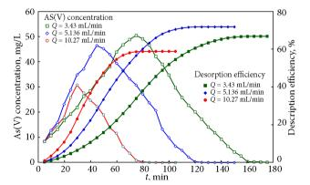
Figure 13. Effect of flow rate on the As(V) desorption efficiencies (eluent concentration: 0.1 mol/L NaOH; adsorbent mass: 2 g; adsorbent grain size: <100 mesh; operating temperature: 35 °C)
