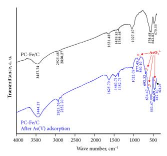
Figure 2. FT-IR spectra of the PC-Fe/C adsorbent prepared with eucalyptus wood biotemplate
