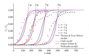
Figure 7. Effect of adsorbent mass on breakthrough curve for As(V) adsorption removal by the PC-Fe/C adsorbent prepared with eucalyptus wood template (influent As(V) concentration: 20 mg/L; flow rate: 5.136 mL/min; pH: 3; adsorbent grain size: <100 mesh; operating temperature: 35 °C)
