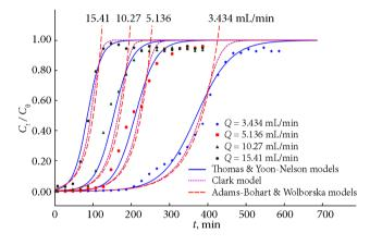
Figure 5. Effect of influent flow rate on breakthrough curve for As(V) adsorption removal by the PC-Fe/C adsorbent prepared with eucalyptus wood template (influent As(V) concentration: 20 mg/L; pH: 3; adsorbent mass: 2 g; adsorbent grain size: <100 mesh; operating temperature: 35 °C)
