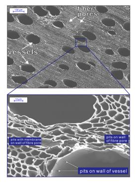
Figure 3. SEM result of the PC-Fe/C adsorbent prepared with eucalyptus wood biotemplate
