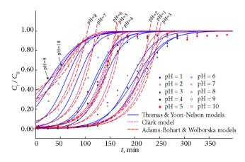
Figure 6. Effect of influent pH on breakthrough curve for As(V) adsorption removal by the PC-Fe/C adsorbent prepared with eucalyptus wood template (influent As(V) concentration: 20 mg/L; flow rate: 5.136 mL/min; adsorbent mass: 2 g; adsorbent grain size: <100 mesh; operating temperature: 35 °C)
