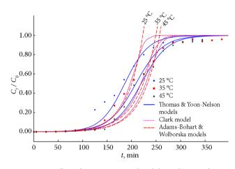
Figure 9. Effect of temperature on breakthrough curve for As(V) adsorption removal by the PC-Fe/C adsorbent prepared with eucalyptus wood template (influent As(V) concentration: 20 mg/L; flow rate: 5.136 mL/min; pH: 3; adsorbent mass: 2 g; adsorbent grain size: <100 mesh)
