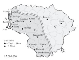
**Fig. 4.** Weather stations with the records of hurricane and catastrophic winds as well as proposed hurricane wind regions A, B, and C
