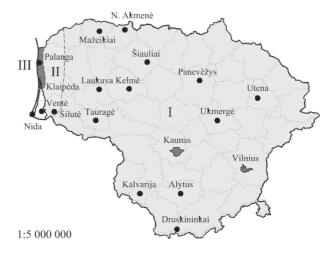
Fig. 5. The map of basic reference wind speeds  $v_{ref,d}$  specified in the design code STR 2.05.04:2003 (see also Table 2)
