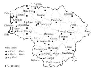
**Fig. 1.** Map showing the network of Lithuanian weather stations with 10-min wind speeds of at least 30 m/s recorded in 1962–2005 (the geographic coordinates of the stations were provided by Lithuanian Hydrometeorological Service, http://www.meteo.lt/)
