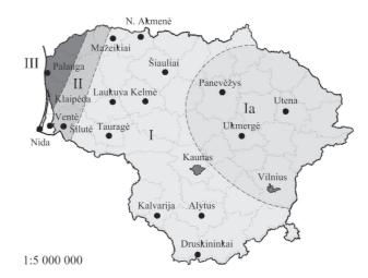
**Fig. 6.** The map of characteristic wind pressures  $w_0$  specified in the design code SNiP 2.01.07-85 (see also Table 3)
