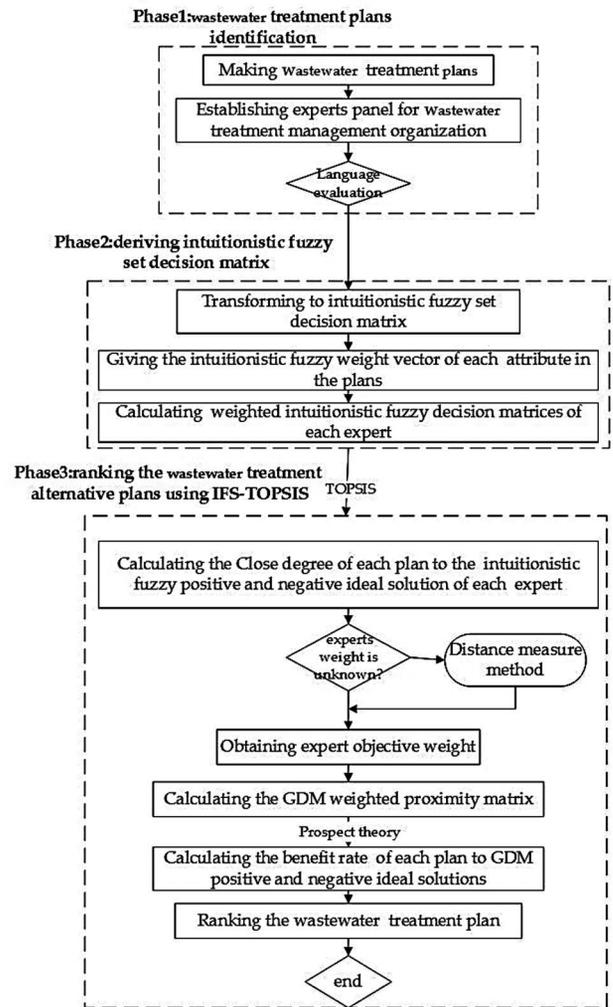
Figure 1. IF-TOPSIS Model for wastewater treatment plans selection
