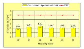
**Fig 13**. Distribution of dust concentrations at Terminal of Powdery Manure Discharge in zone II
