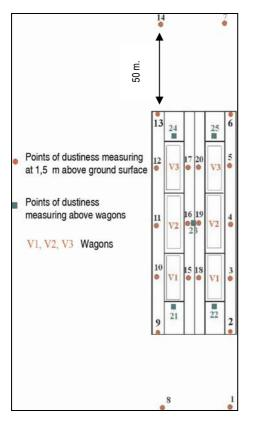
**Fig 2**. Points of measuring dustiness at Terminal of Powdery Manure Discharge
