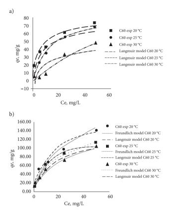
Figure 5. Langmuir 4 and Freundlich non-linear adsorption isotherms of BPA on C 60; Conditions: Ci = 10-50 mg/L BPA, t = 20, 25, 30 °C, V = 100 mL, 0.1 M NaCl (a) and 0.01 M NaCl (b), contact time 3 hours, equilibrium reached after 30 minutes
