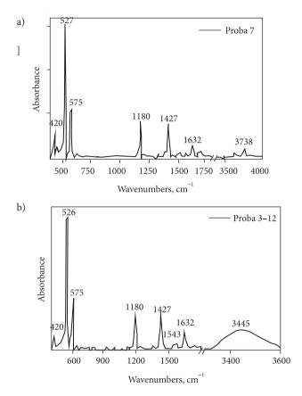
Figure 2. FTIR spectra of simple and impregnated nanostructures, a) C60 without BPA, b) C60 with BPA
