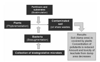
**Fig 1.** Principal scheme of technological approach for remediation of oil-shale chemical industry solid waste dump area
