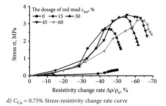
Figure 5. Curves of stress-strain, and stress-resistivity change rate of 28 d solidified soil
