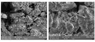
a) 3000 × b) 10000 × Figure 2. Microscopic morphology of loess particles
