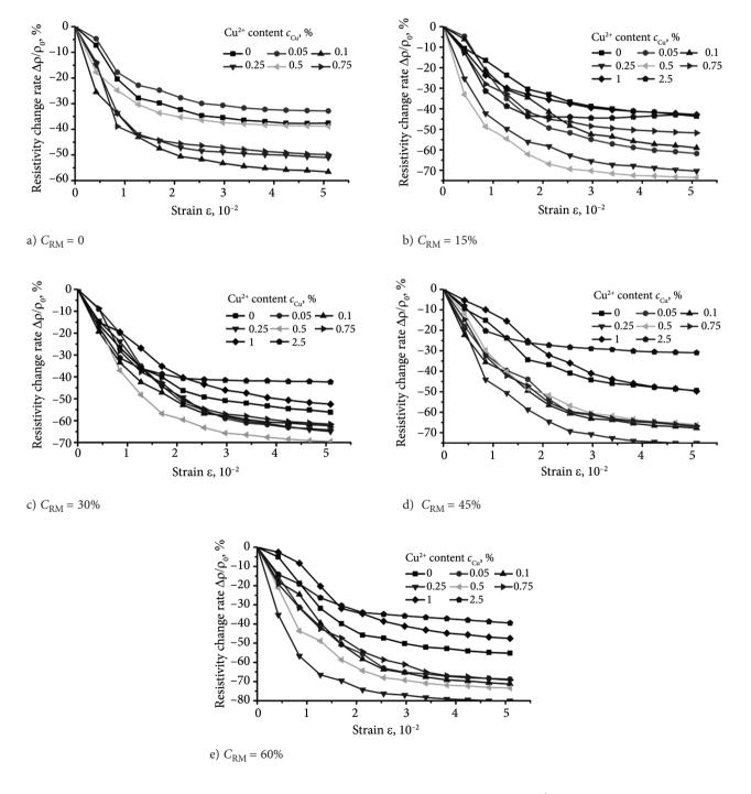
Figure 8. Curves of resistivity change rate and strain of solidified soil with different Cu<sup>2+</sup> contents after 28 days
