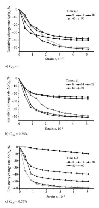
Figure 9. Relation of resistivity change rate and strain of solidified soil at different curing ages
