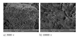
Figure 3. Microscopic morphology of red mud particles
