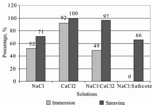
**Fig. 3.** Percentage rate of carbon steel corrosion product cover by immersion and spraying methods
