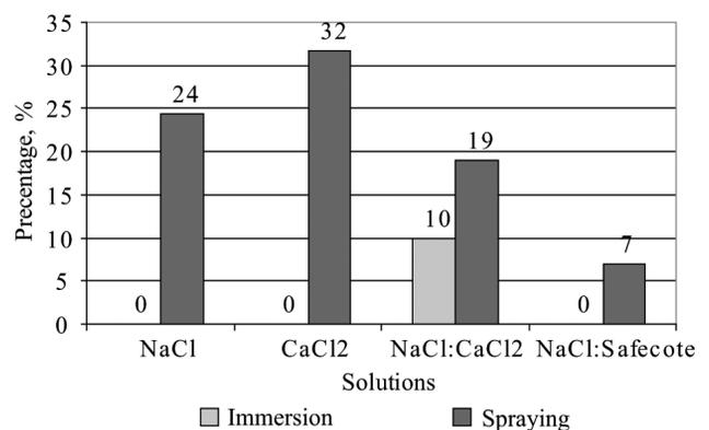
**Fig. 4.** Percentage rate of stainless steel corrosion product cover by immersion and spraying methods
