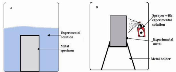
**Fig. 1.** Laboratory experiments. A – Immersion method; B – Spraying method
