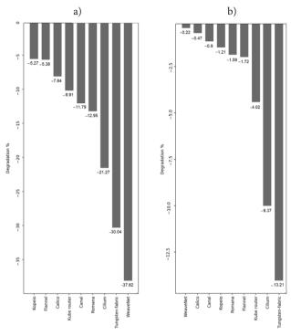
Figure 4. CNI plugins application layer protocol HTTP relative trhoughput degradation in virtual environment (a) 1500MTU (b) 9000B MTU
