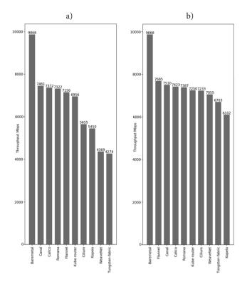
Figure 2. CNI plugins TCP protocol throughput comparison to bare matal results in (a) virtualized environment and (b) physical environment for 1500B MTU
