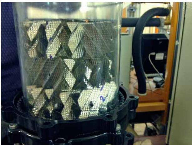
Fig. 14. Short layered packing in the column apparatus
