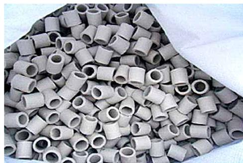
Fig. 4. Ceramic Raschig rings
