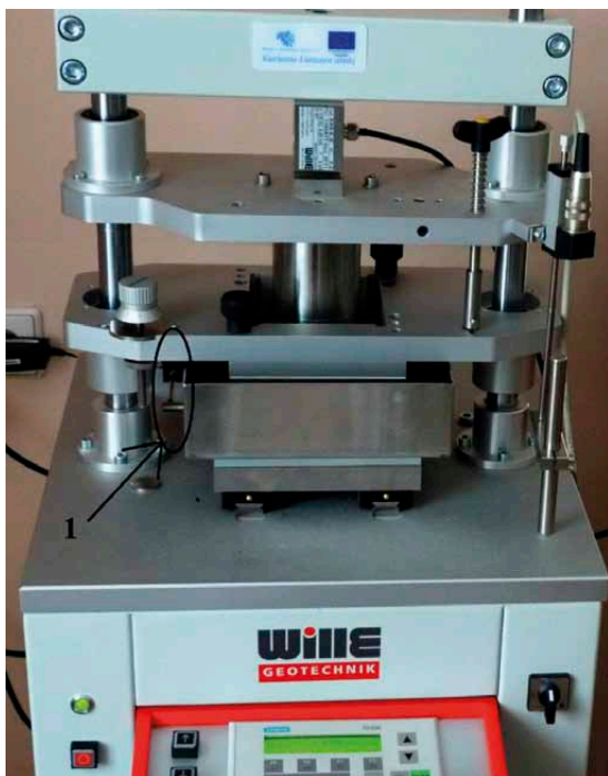
Fig. 3. Direct shear apparatus. 1 – external horizontal displacement transducer
