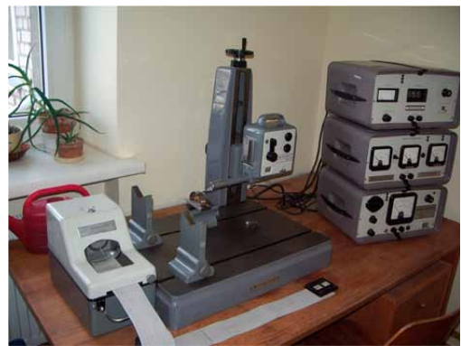
5 pav. Profilometras-profilografas TALYSURF 4 Fig. 5. Roughness meter TALYSURF 4
