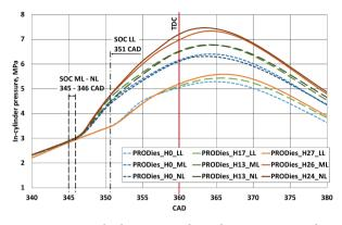
Figure 4. In-cylinder pressure dependence on CAD and position of SOC at various loads and HES with PRO Diesel
