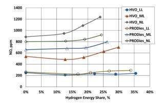
Figure 9. The dependence of NO on the load and HES
