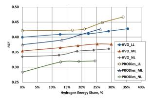
Figure 5. The dependence of BTE on fuel used, loads and HES
