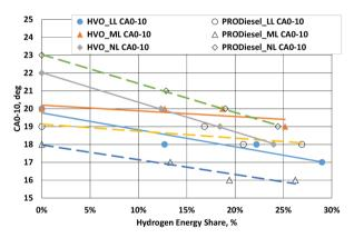
Figure 11. The combustion delay of 0–10% MFB at tested HES of HVO and PRO Diesel
