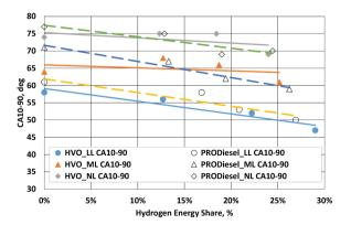
Figure 12. The combustion delay of 10–90% MFB at tested HES of HVO and PRO Diesel
