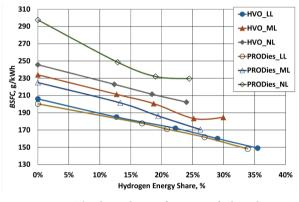
Figure 6. The dependence of *BSFC* on fuel used, loads and HES
