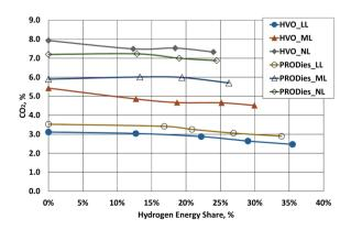
Figure 8. The dependence of CO<sub>2</sub> on fuel used, loads and HES
