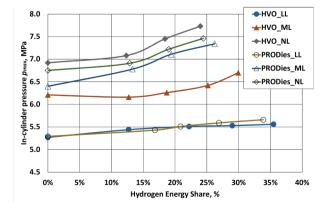
Figure 2. In-cylinder max pressure  $p_{max}$  at Low, Medium and Nominal Loads and HES
