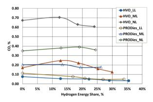
Figure 7. The dependence of CO on fuel used, loads and HES
