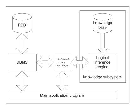
Figure 5. Conceptual architecture of the quality inspection system.
