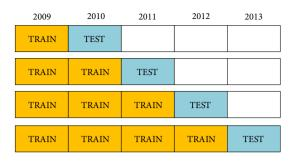
Figure 1. An illustration of out-of-time validation
