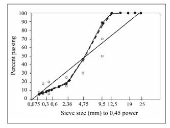
**Fig 4.** Aggregate gradations for all test series (up-limit and down-limit)
