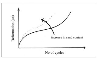
Fig 2. Permanent deformation of a mix
