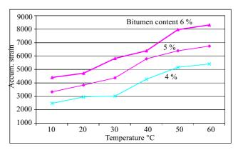
Fig 6. Effect of bitumen content and temperature on accumulated strain  $(\mu\epsilon)$
