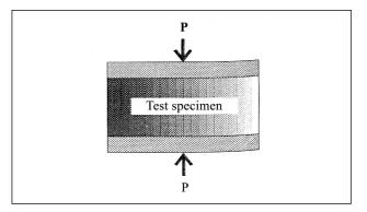
Fig 3. Specimen setup for permanent compressive strain test
