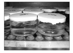
**Fig 1.** The samples used for determining the water vapour permeability in the paint-thin rendering system
