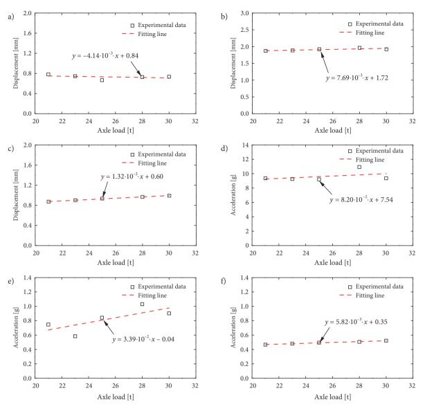
Figure 13. Statistical results as increase of train running speed: a – rail lateral displacement; b – rail vertical displacement; c – sleeper vertical displacement; d – rail vertical acceleration; e – sleeper vertical acceleration; f – ballast bed vertical acceleration variation with increasing axle load
