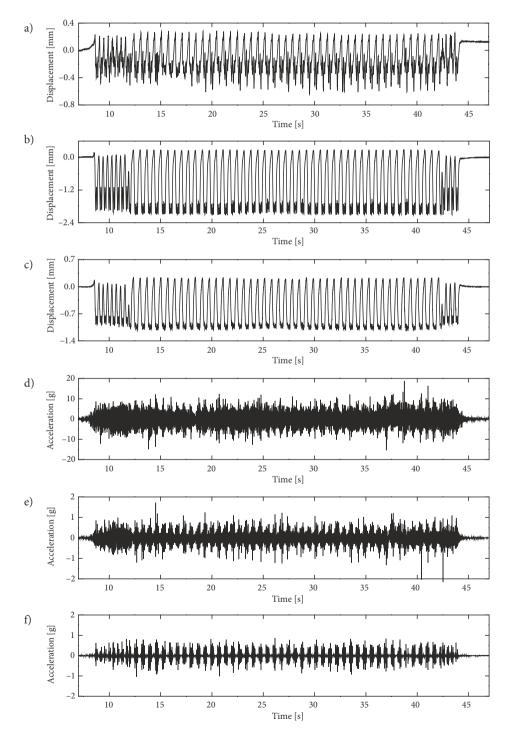
Figure 9. Time histories of the track vibration: a – rail lateral displacement; b – rail vertical displacement; c – sleeper vertical displacement; d – rail vertical acceleration; e – sleeper vertical acceleration; f – ballast vertical acceleration
