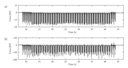
Figure 8. Time histories of wheel-rail dynamic force: a - lateral; b - vertical
