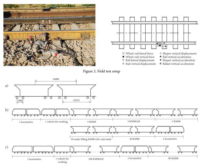
Figure 3. Formations of the test trains: a - characteristic lengths of KM98 vehicle; b - 5400 t test train; c - 23000 t test train
