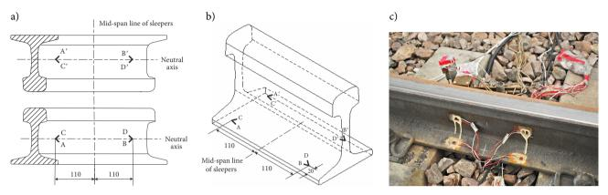
Figure 4. Wheel-rail dynamic force test scheme: a - strain gauge arrangement for vertical force measurement; b - strain gauge arrangement for lateral force measurement; c - photo of the field testing
