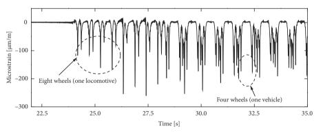
Figure 7. Microstrain signal representing the wheel-rail vertical dynamic forces
