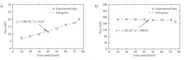
Figure 10. Variations of the peak values of the wheel-rail force with train running speed: a - lateral; b - vertical
