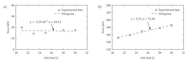
Figure 12. Variations of the peak values of the wheel-rail force with axle load: a - lateral; b - vertical
