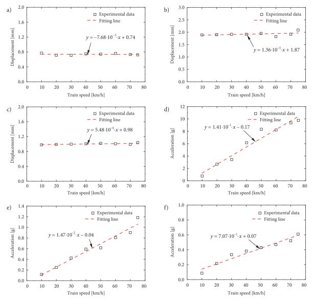
Figure 11. Statistical results as increase of train running speed: a – rail lateral displacement; b – rail vertical displacement; c – sleeper vertical displacement; d – rail vertical acceleration; e – sleeper vertical acceleration; f – ballast bed vertical acceleration vary with train speed increasing
