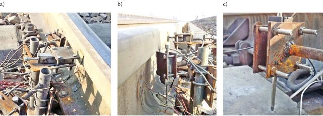
Figure 5. Arrangement of displacement sensors along: a - rail lateral direction; b - rail vertical direction; c - sleeper vertical direction
