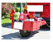
Figure 2. Single-wheel dynamometer trailer
