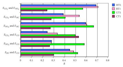
Figure 20. Coefficient of Spearman's rank correlation R between the emission intensity of specific pollutants  $(E_{CO_2}, E_{NO_X}, E_{CH}, E_{CO})$  in individual tests (CT1, UT1, RT1, HT1)
