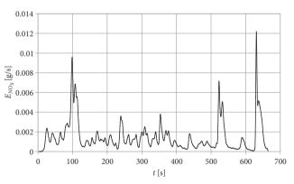
Figure 13. Time history of the nitrogen oxides emission intensity  $E_{NOx}$  in the CT1 test
