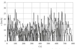
Figure 1. CT test (stochastic process of vehicle speed) for street congestions
