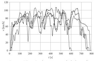
Figure 3. RT test (stochastic process of vehicle speed) for extra-urban (rural) traffic
