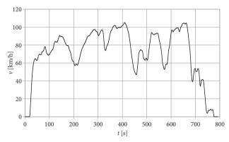
Figure 8. Vehicle speed v vs. time t curve in the RT1 test
