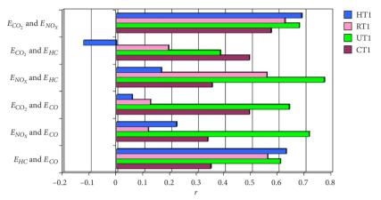
Figure 19. Coefficient of Pearson's linear correlation r between the emission intensity of specific pollutants  $(E_{CO_2}, E_{NO_X}, E_{CH}, E_{CO})$  in individual tests (CT1, UT1, RT1, HT1)
