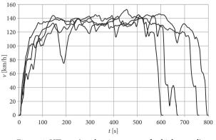
Figure 4. HT test (stochastic process of vehicle speed) for motorways and fast roads
