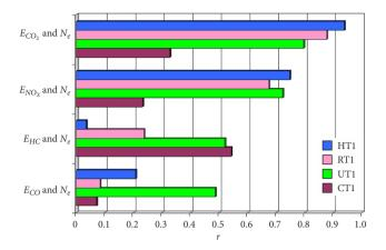
Figure 15. Coefficient of Pearson's linear correlation r between the pollutant emission intensity ( $E_{CO_2}$ ,  $E_{NO_X}$ ,  $E_{CH}$ ,  $E_{CO}$ ) and the non-negative effective power of the engine  $N_e$ in individual tests (CT1, UT1, RT1, HT1)
