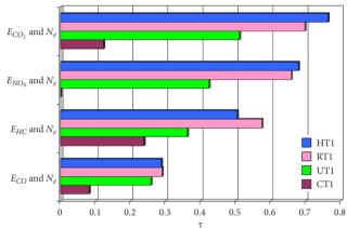
Figure 18. Coefficient of Kendall's tau correlation  $\tau$  between the pollutant emission intensity ( $E_{CO_2}$ ,  $E_{NO_X}$ ,  $E_{CH}$ ,  $E_{CO}$ ) and the non-negative effective power  $N_e$  in individual tests (CT1, UT1, RT1, HT1)
