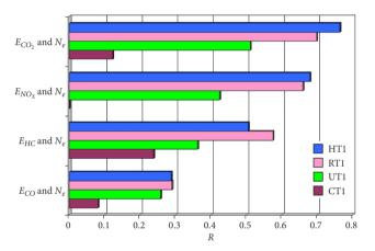
Figure 16. Coefficient of Spearman's rank correlation *R* between the pollutant emission intensity  $(E_{CO_2}, E_{NO_X}, E_{CH}, E_{CO})$ and the non-negative effective power  $N_e$  of the engine in individual tests (CT1, UT1, RT1, HT1)
