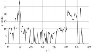
Figure 6. Vehicle speed v vs. time t curve in the CT1 test
