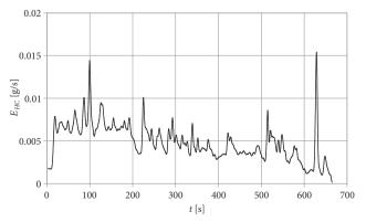
Figure 12. Time history of the hydrocarbons emission intensity  $E_{CH}$  in the CT1 test
