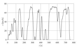
Figure 7. Vehicle speed v vs. time *t* curve in the UT1 test
