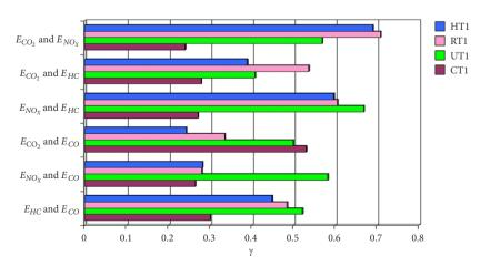
Figure 21. Coefficient of Kruskal's gamma correlation  $\gamma$  between the emission intensity of specific pollutants ( $E_{CO_2}$ ,  $E_{NO_X}$ ,  $E_{CH}$ ,  $E_{CO}$ ) in individual tests (CT1, UT1, RT1, HT1)
