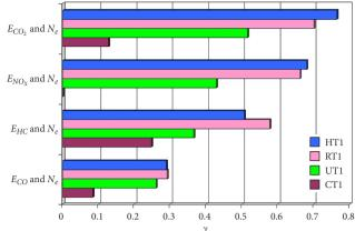
Figure 17. Coefficient of Kruskal's gamma correlation  $\gamma$  between the pollutant emission intensity ( $E_{CO_2}$ ,  $E_{NO_x}$ ,  $E_{CH}$ ,  $E_{CO}$ ) and the non-negative effective power  $N_e$  in individual tests (CT1, UT1, RT1, HT1)
