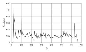
Figure 11. Time history of the carbon monoxide emission intensity  $E_{CO}$  in the CT1 test
