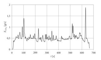
Figure 14. Time history of the carbon dioxide emission intensity  $E_{CO_2}$  in the CT1 test
