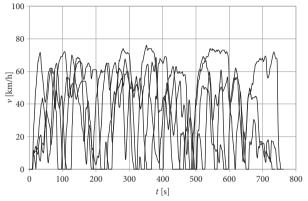
Figure 2. UT test (stochastic process of vehicle speed) for urban traffic without congestions
