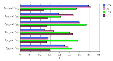
Figure 22. Coefficient of Kendall's tau correlation  $\tau$  between the emission intensity of specific pollutants  $(E_{CO_2}, E_{NO_3}, E_{CH}, E_{CO})$  in individual tests (CT1, UT1, RT1, HT1)
