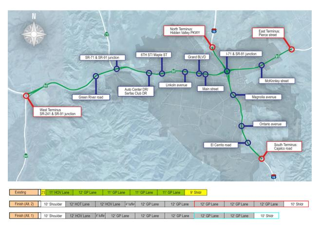
Figure 2. SR-91/I-15 project vicinity map and pavement cross-sections (\*Alt. 1 represents Alterative A and Alt. 2 represents Alternative B; both represent the section from SR-71 to I-15)
