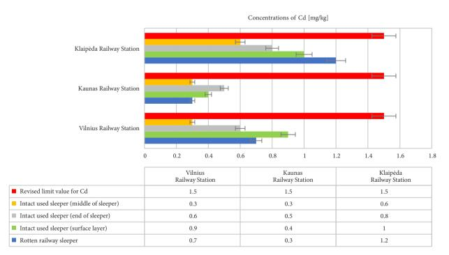
Figure 6. The distribution of the concentrations of Cd in the intact used and rotten wooden railway sleepers at the biggest Lithuanian railway stations (Vilnius, Kaunas and Klaipėda)
