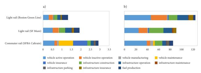
Figure 2. Total energy consumption (a) in [MJ/pkm] and total  $CO_{2e}$  emission (b) in  $[g CO_{2e}/pkm]$  of selected rail transport (redrawn by use of data from Chester and Horvath (2009))
