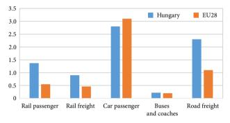
Figure 9. Safety total impacts performance index, i.e. external costs generated by the safety impacts in year 2014 (the costs induced by congestions are excluded) ([€ ct/pkm] and [€ ct/0.1 tkm])
