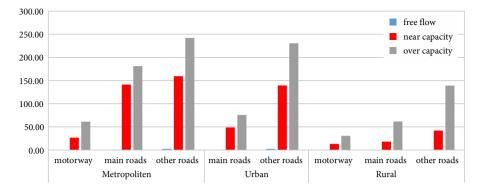
Figure 7. Congestion cost [€ ct/vkm] recommended to apply by Quddus et al. (2010)
