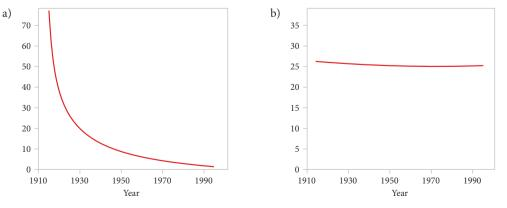
Figure 3. Changes in road transport safety indicators depending on proportion to different basis: a – death in traffic accidents per 100 million miles driven; b – death in traffic accidents per 100 thousand registered drivers (redrawn by use of data from CORDIS (2006))
