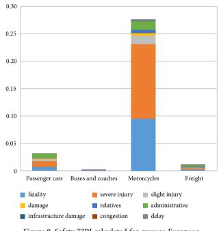
Figure 8. Safety TIPI calculated for average European road transport for year 2014 (in [€/pkm] and [€/1 tkm] for freight transport)
