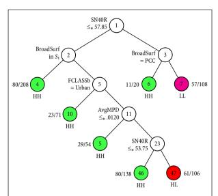
GUIDE classification tree with estimated priors and unit misclassification costs. At each intermediate node, an observation goes to the left branch if and only if the condition is satisfied. The symbol ' $\leq_*$ ' denotes ' $\leq$  or missing'. Set  $S_1 = \{PCC, SMA\}$ . Predicted classes (based on estimated misclassification cost) below terminal nodes; #misclassified/sample size beside each node.
