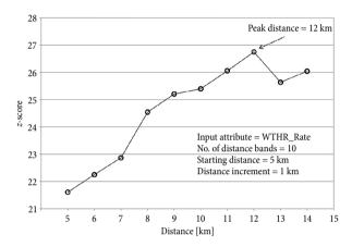
Fig. 1. Result of Global Moran's *I* statistic showing distance bandwidth of peak clustering of weather-related crash rate in Wisconsin
